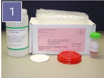
1) Fiberboard Shipper; Red-topped Secondary Container (95kPa container); Protective Bubble Wrap; absorbent pad; Primary Container.
